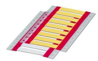
Marker for thermal transfer printer, unperforated, white, labeling field: 50 x 5 mm, can be used for 2.4 mm diameter, shrinkage ratio 3:1, 1 roll = 500 Marker, 1 roll = 250 Marker at 50 mm
